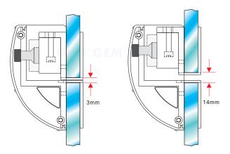
The armature plate can be adjusted depends on the door gap between door and lock, with only  $3\,\text{mm}{\sim}14\,\text{mm}$  width of the door gap.
